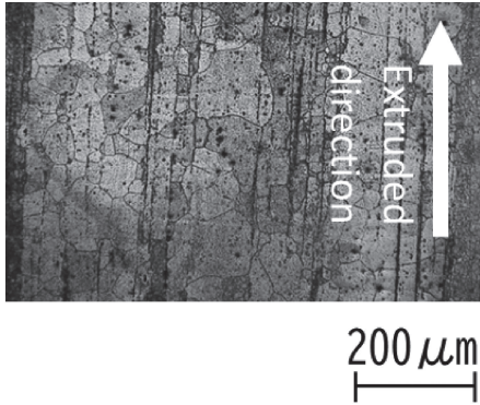
Fig. 1 Initial microstructure of the Mg–Li–Al–Ca alloy.
